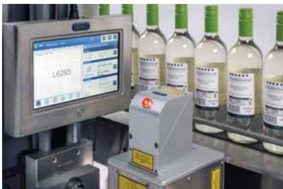
Laser marking system on a wine bottling line
