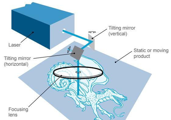
These systems write like a pen. The first systems, based on pulsed Nd:YAG lasers, were introduced in 1969. Systems using Continuous Wave (CW) CO<sub>2</sub> lasers were not introduced until the early 1980s. But in the first years this principle was rarely used, as the mirrors for each direction need a very fast and robust control algorithm that could only be realised with high performance signal processors.
