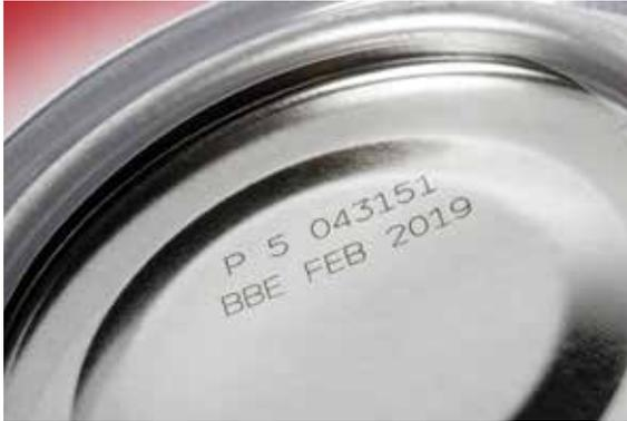
Fibre laser marking on bare metal
