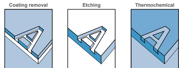
These marks look similar to an embossed print. On glass the laser induces thermal stress, causing microcracks in the surface and resulting in tiny glass crystals being ejected from the surface to produce a mark.
